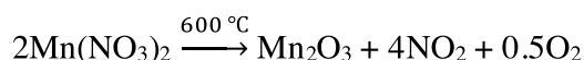
Scheme 1. The oxidation of manganese ions from Mn 2+ (in nitrate salt) to Mn 3+ (in Mn 2 O 3 oxide).
