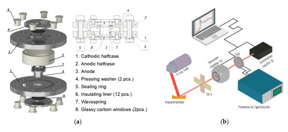
**Figure 1.** (a) Design of the electrochemical cell for laboratory operando XAS studies. (b) Scheme of the experimental setup. The main parts of the laboratory X-ray absorption spectrometer are shown, the cell is installed on the sample position and connected to a potentiostat/galvanostat device.
