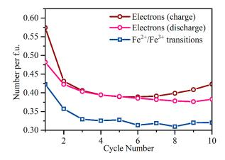
**Figure 5.** The number of electrons per formula unit transferred through the cell upon charge and discharge as derived from experimental electrochemistry data. The blue bottom curve shows the number of  $Fe^{2+}/Fe^{3+}$  redox transitions per formula unit obtained from operando XAS as a function of cycle number.
